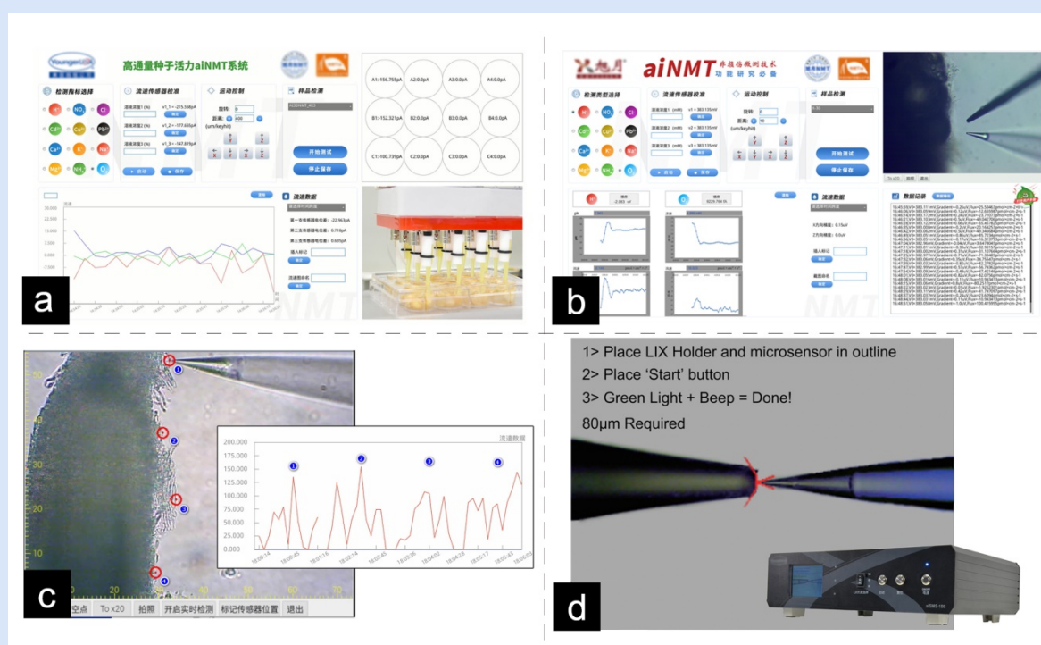
Figure 6. AI's Applications in NMT. Any combinations of any number of NMT ion(s)/molecule(s) microsensors are doable now due to the adoption of AI sampling rules. a: A High-throughput aiNMT System can measure seed vigor in a 12-well plate in a fully automatic fashion; b: A dual-sensor configuration was used to simultaneously measure both H + /O 2 fluxes of a tumor tissue; c: Illustration of AI-based automatic sample image recognition and testing point locating; d: AI-based NMT microsensor making instrument by which a tiny volume (ca. one millionth of a drop of water) of liquid ionophore can be manipulated accurately.
